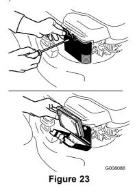
3. Install a new air filter and the air filter cover.
